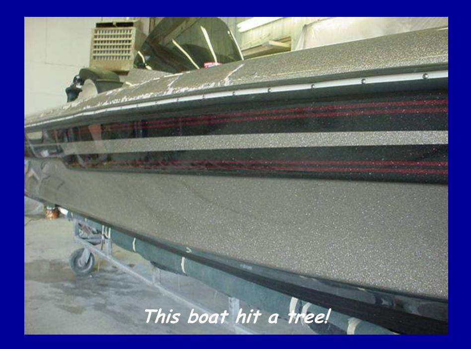
Bad areas cut out and new fiberglass being applied. A lot of work to be done...
